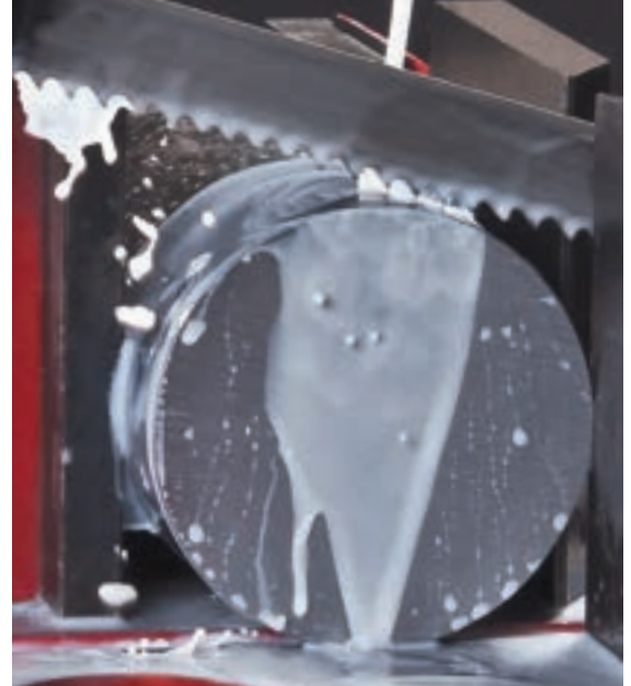
Start to cut material at reduced cutting rate
